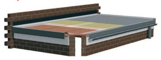
Edge trims are manufactured in GRP. One side has a high adhesion finish (matt finish), the other side has a glossy finish, always bond to the matt finish.
