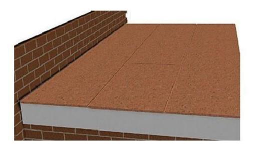
18mm OSB3 boards are laid lengthways at 90° to the roof joists. The boards must be laid with the writing side uppermost. Not only does this give a better key for the laminate, it also allows the resin to flow into the board joint to effectively glue the boards together.
