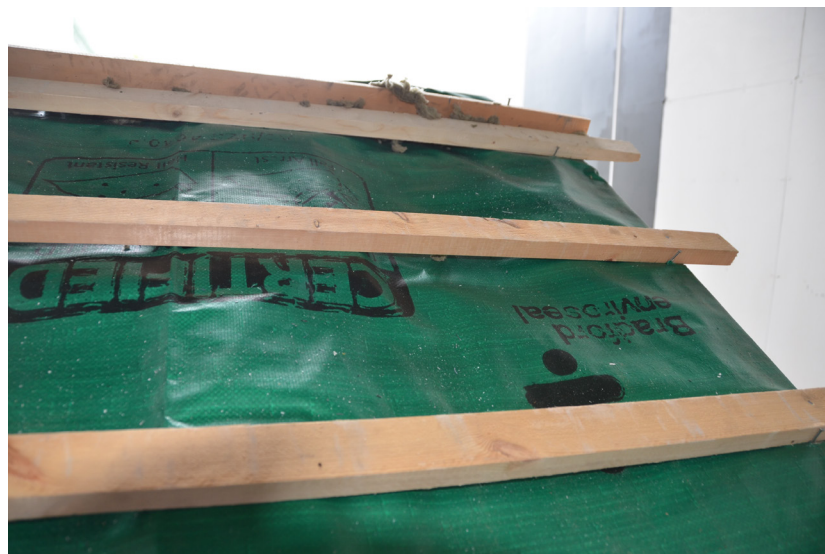
Figure 10. Photograph of sarking placed under terracotta tiles (flat tiles) taken immediately after the experiment was complete. The tiles have been removed. No firebrand penetration was observed.
