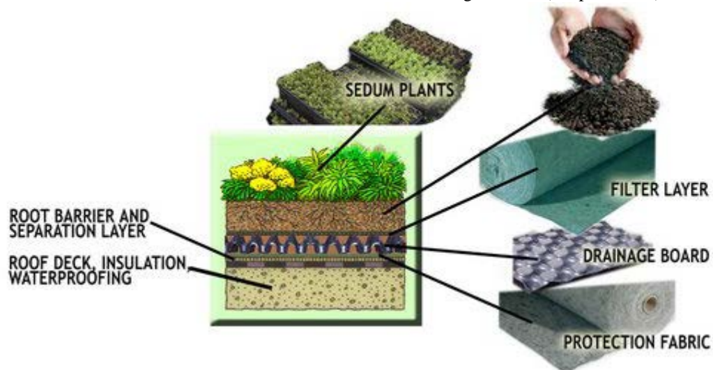
Fig 5: Extensive green roof (Breuning, 2015)
