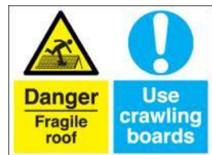
Figure 2: Example of signage to alert workers to fragile roofing material.
