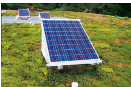
The test involved two modules installed on “naked” bituminous panels being compared with one module installed on a green roof. In each case, attention was focused on the temperature at the underside of the panels.
