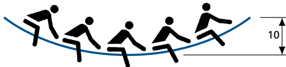
Simply supported span Deflection varies with the position of the load
