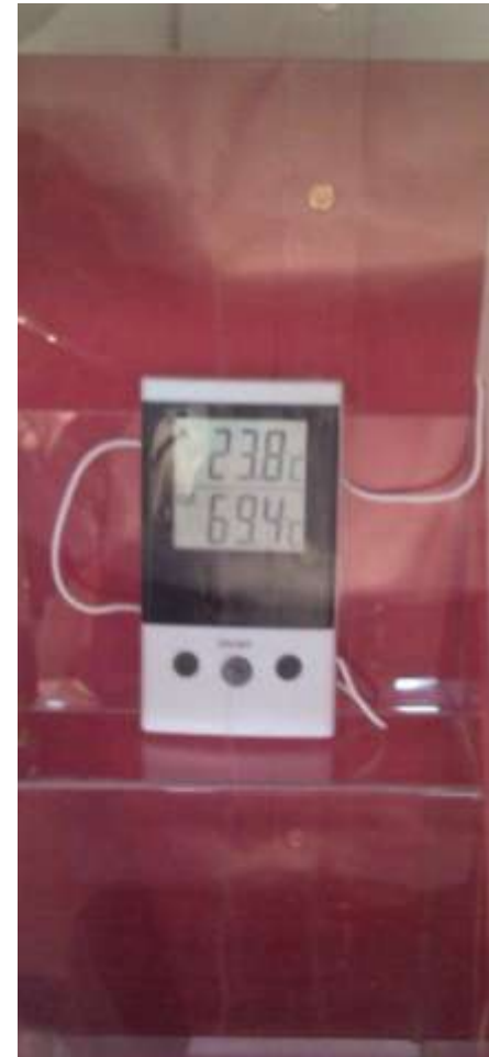
Clay Tiles + Insulator 23.8°C
