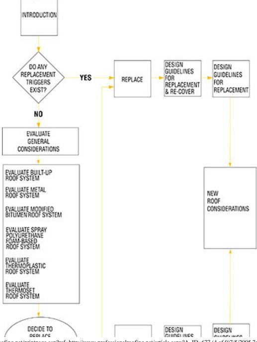
Low-slope reroofing guidelines | July 2005 | Professional Roofing Magazine
