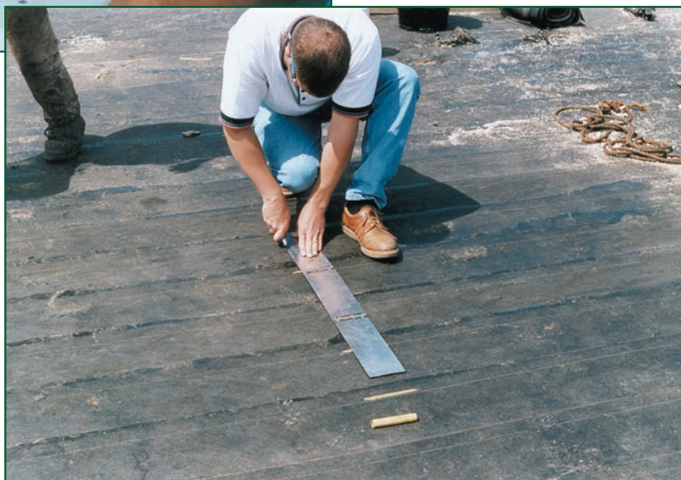
Photo 5: The template is laid perpendicular to the shingle sequence, across the limits of the sample area.
