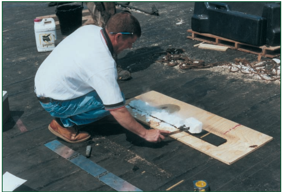
Photo 8: Covering the removed sample with a blanket of dry ice prior to separating the felts.
